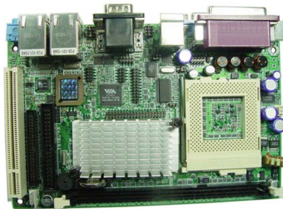
NASA-6822 Low Power 1GHz EBX board
